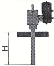
Dimension H should be smaller than dimension X, so that the pump pipe does not reach the drum bottom.
