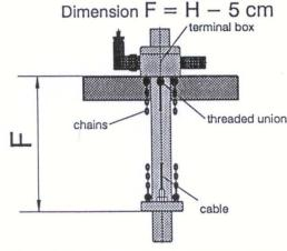
Dimension F must be smaller than dimension H in order to prevent the pump from taking in any air when it is going to be emptied
