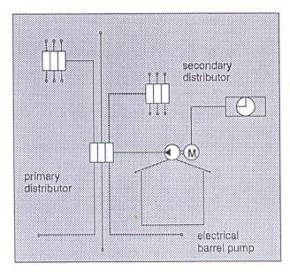
By means of the electrical barrel pump, the lubricant is fed directly into the primary (master)
