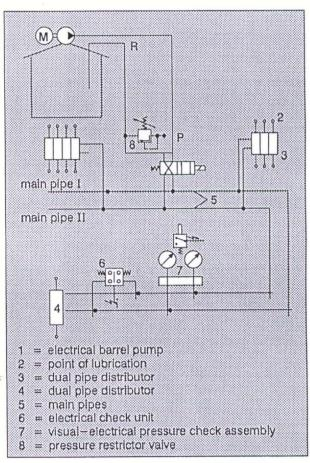
The dual pipe system comprizes two main pipes which are pressurized by alternating sequence of operation, by means of a valve, thus being able to supply lubricant to the dual pipe distributors concerned. Subsequently, the dual pipe distributor supplies the required quantity of lubricant (pre—set at the distributor) to the points of lubrication concerned.
