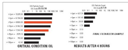
Results shown are subject to variations according to system size, flow rate, and original oil condition
