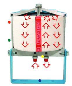
The high tech cartridge gives continuous all round protection against water and ultra-fine debris with contaminated oil entering the filtakleen unit at the base flowing up the centre tube through the 1 micron filter before flowing back to the hydraulic circuit. Flow rates through filter 4.1 I/min to 6.1 I/min depending on unit fitted
